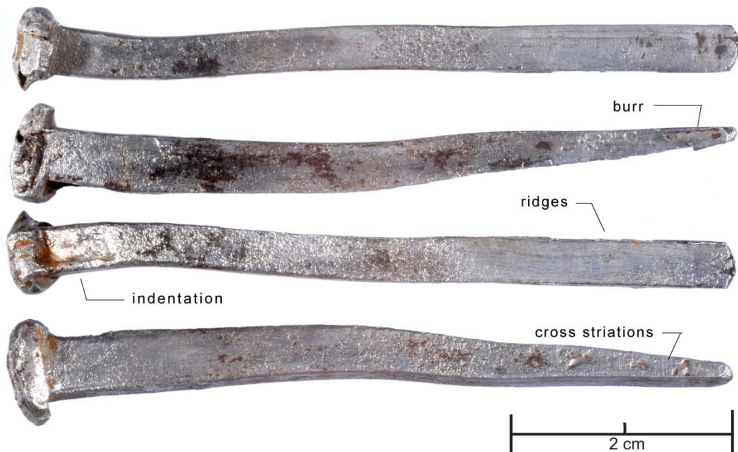
Photograph 31 Cut and rolled Type 3 machine made nail from Pontville ceiling, 1844-45
