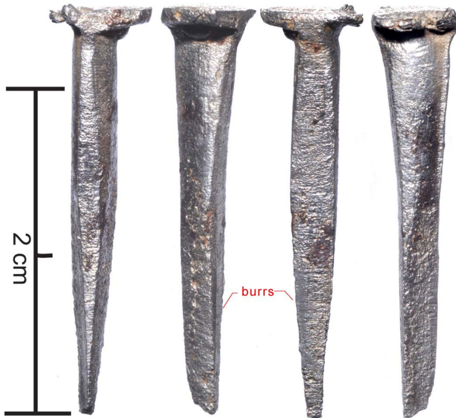
Photograph 33 Lath tack from Pontville ceiling joist with manufacture marks, Type 1. Installed in 1843-44
