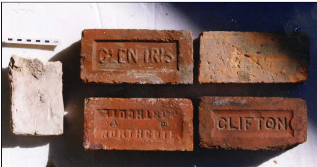
Photograph 40 These are the five types of bricks found at Pontville. The orange brick, upper right is the hand-made Pontville brick and the white cream coloured brick on the left is also hand-made and was incorporated in the Pontville original construction. Scale in centimetres.
