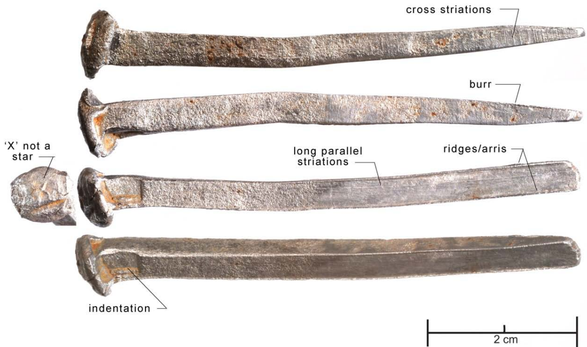
Photograph 30 Cut and rolled Type 3 machine-made nail from Pontville ceiling, mark (inset), 1844-1845.
